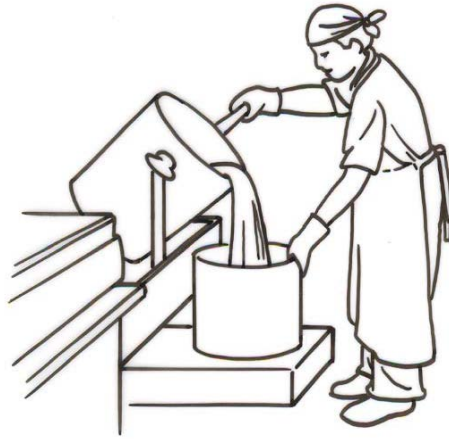
Figure 56.37 Self height-adjusting storage container that turns
