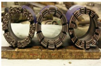
**Figure 5: Diamond Drill Bits**
