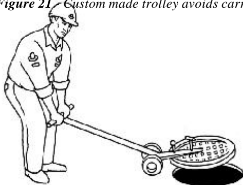
Figure 21 - Custom made trolley avoids carrying.
