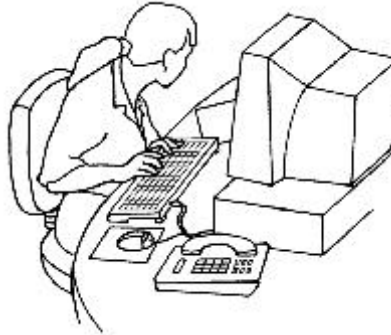
Figure 64 - Poor placement of documents while keyboarding can lead to awkward postures.
